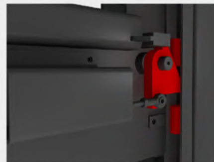
Mechanical anti-falling lock device to protect machine all the way
